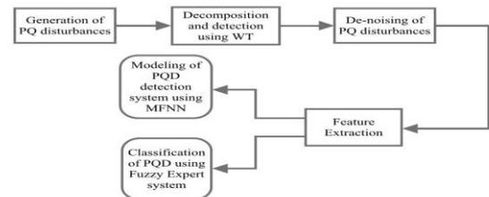
Figure 1 Block Diagram of the method adopted
