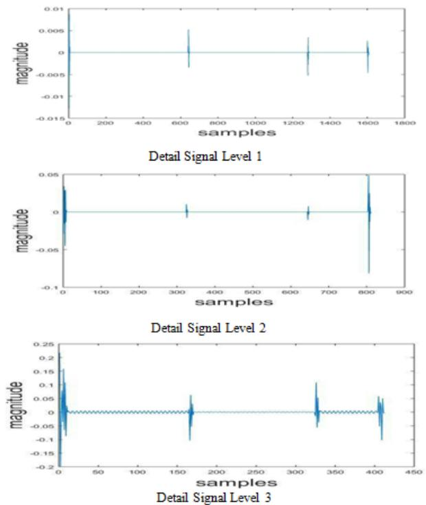
FIG 6 Decomposition of voltage sag
