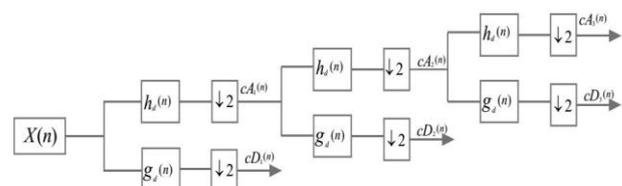
Figure 2 Decomposition Algorithm
