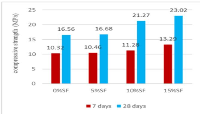
Fig.2 Graph showing compressive strength (MPa) cured at 150°C in oven
