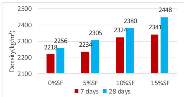
Fig.7 Graph showing density of cylinders cured at 90°C in oven
