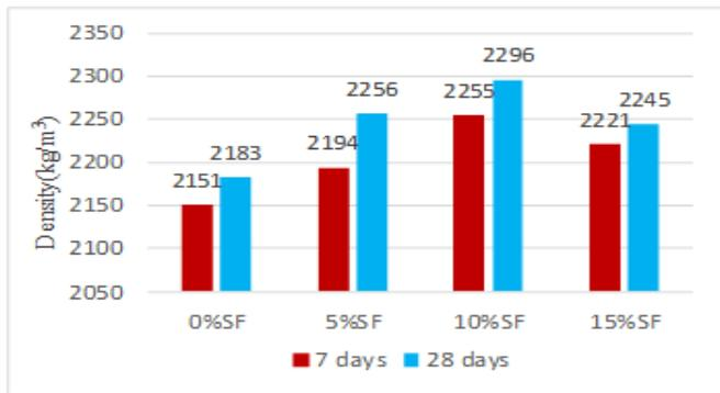
Fig.5 Graph showing density of cubes cured at 90°C in oven
