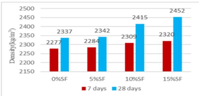
Fig.6 Graph showing density of cubes cured at 150°C in oven
