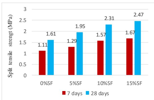
Fig.3 Graph showing Split tensile Strength (MPa) cured at 90°C in oven
