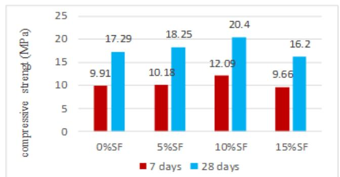
Fig.1 Graph showing compressive Strength (MPa) cured at 90°C in oven
