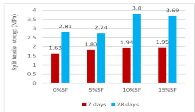
Fig.4 Graph showing Split tensile Strength (MPa) cured at 150°C in oven.
