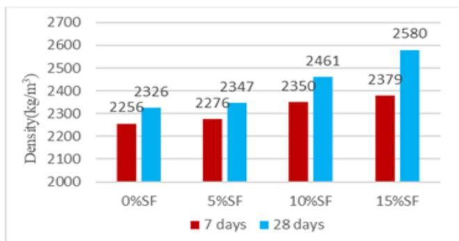
Fig.8 Graph showing density of cylinders cured at 150°C in oven
