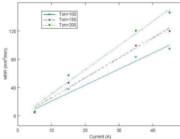
*Fig-1: Material Removal rates with varying current conditions for Experiment.*
