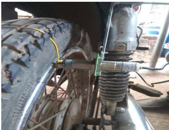
Fig -2: Fabricated Proximity Sensor on rear wheel
