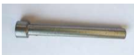
Fig.7 TiAlN coated pin
