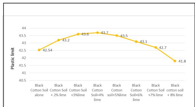
Chart -5: Plastic limit of BCS with various percentage of lime after seven days curing.
