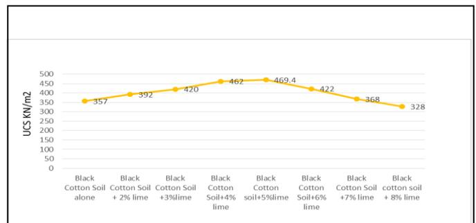
**Chart -7:** Immediate results of Unconfined Compressive Strength of BCS treated with various percentage of lime.
