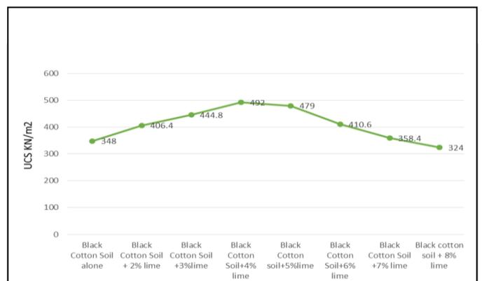
**Chart -8:** Unconfined Compressive Strength of BCS treated with various percentage of lime after seven days curing.
