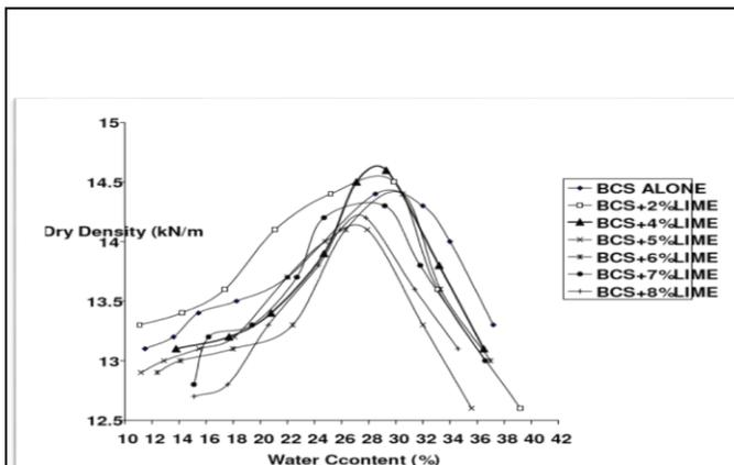
**Chart -6:** Compaction behavior of lime treated Black cotton soil with various percentage of lime.
