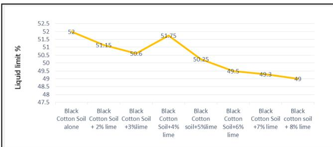
Chart -3: Liquid limit of BCS with various percentage of lime after seven days curing.
