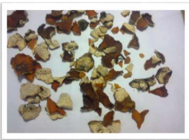
Fig- 1: Dry Orange Peels for Adsorbent
