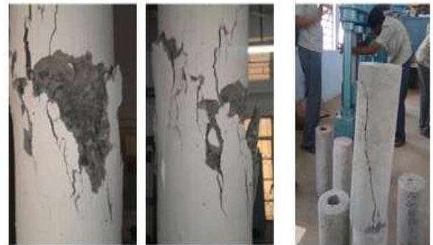
Figure 4: Failure pattern for Conventional Column
