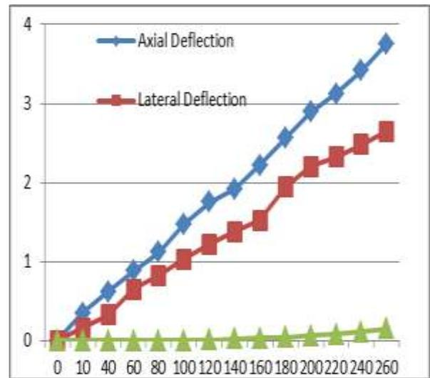
Figure 7: Load and Deflection Behavior of Solid RCC Column
