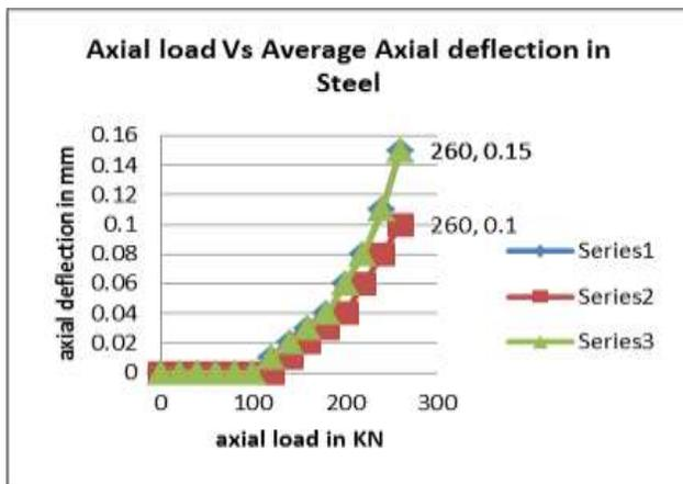
Figure 12: Axial load Vs Average Axial deflection in Steel
