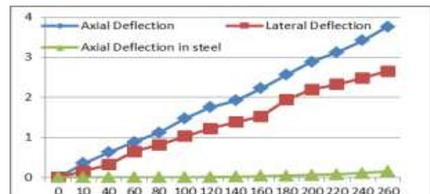
Figure 9: Load and Deflection Behavior of Conventional Hollow RCC Column confined with External FRP Jacketing
