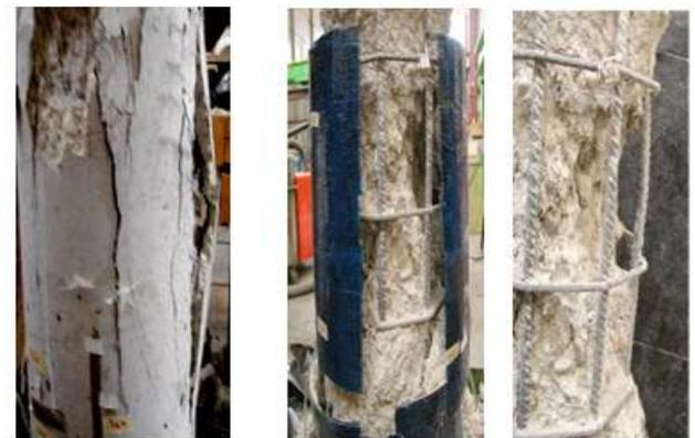
Figure 5: Failure pattern for Solid Column
