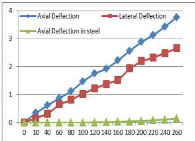
Figure 8: Load and Deflection Behavior of Hollow RCC Column
