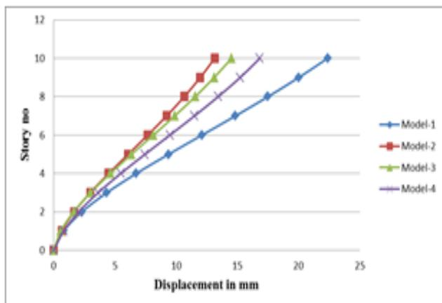
Fig 4.2: Story Displacement by ESA along Y- Direction
