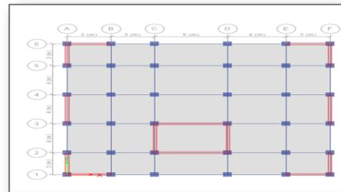
Fig 1-Plan view of flat plates with shear wall
