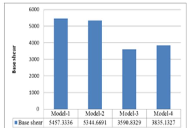
Fig 4.5: Base Shear by ESA along X-Direction
