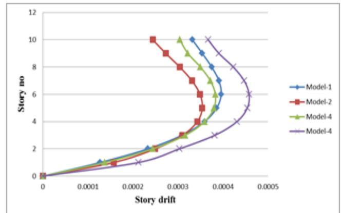
Fig 4.10: Story Drift by RSA along Y-Direction
