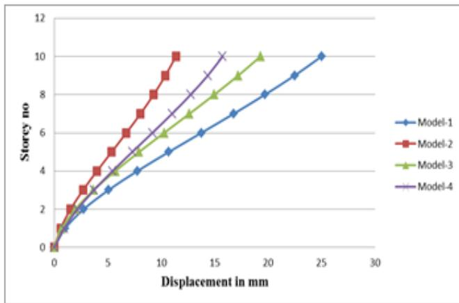
Fig 4.1: Story Displacement by ESA along X- Direction
