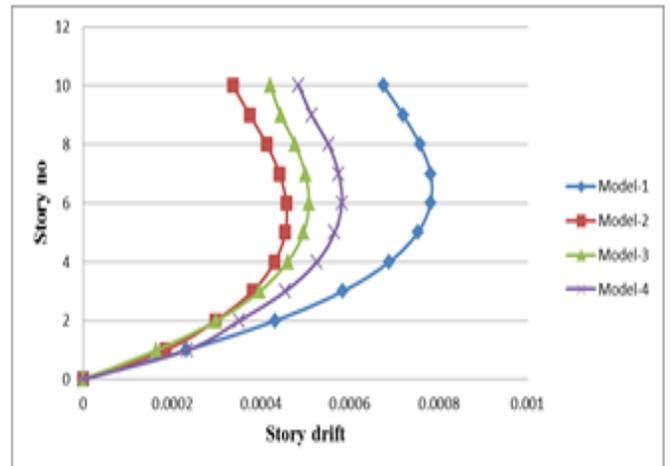
Fig 4.4: Story Drift by ESA along Y-Direction
