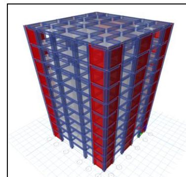
Fig 2- 3D view of flate plate with shear wall
