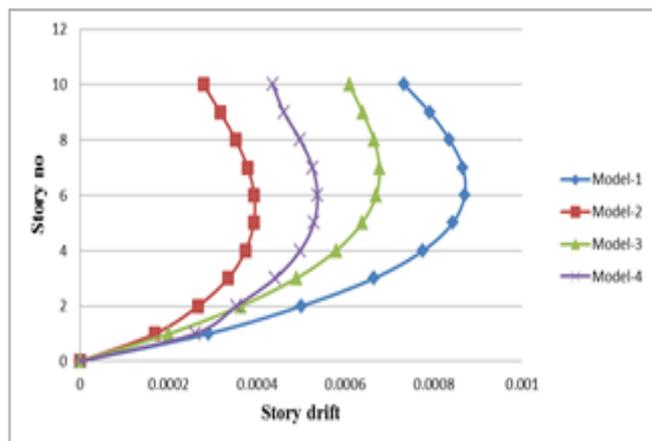
Fig 4.3: Story Drift by ESA along X-Direction
