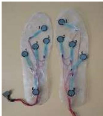
Fig -2: FSR position at Hallux (1), Medial forefoot (2), Central forefoot (3), Lateral forefoot (4), and Heel (5).
