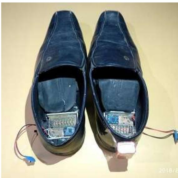
Fig -3: Hardware installed in heel of the shoes.
