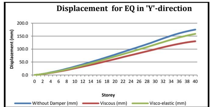
**Chart -2:** Displacement for Earthquake load applied in 'Y'-direction
