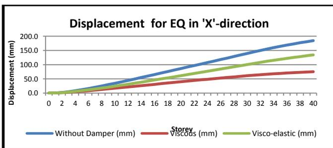
**Chart -1:** Displacement for Earthquake load applied in 'X'-direction
