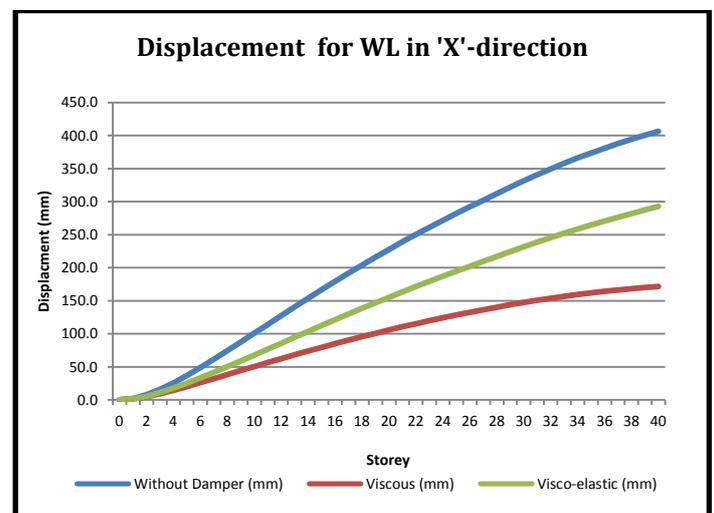
**Chart -3:** Displacement for Wind load applied in 'X'-direction
