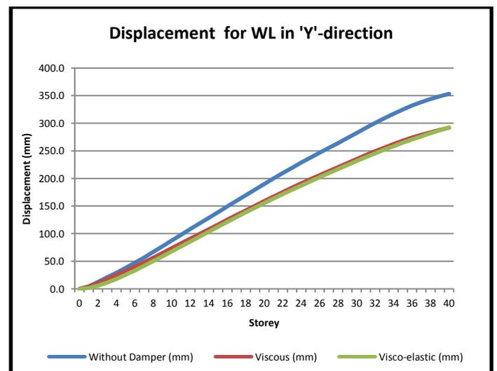
**Chart -4:** Displacement for Wind load applied in 'Y'-direction
