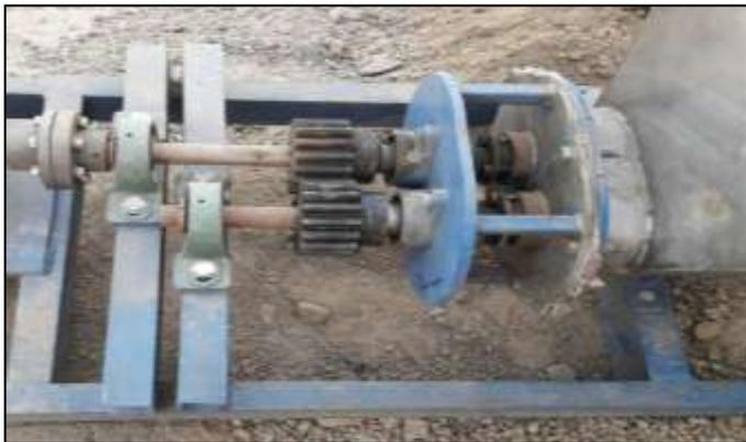
Fig 3 -: Gears used in the machine
