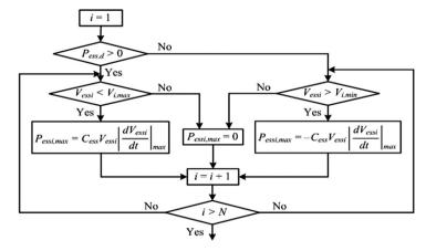
Fig. 4.1. Flowchart of determination of Pessi, maxfor each WTG.
