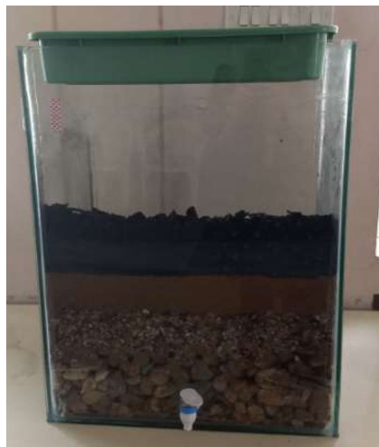
Fig. 2.3: Filter Model Using Natural Materials
