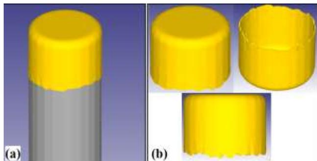
Fig -5: FE simulation of reversely deep-drawn cup (2nd stage); (a) formed cup, (b) different views.
