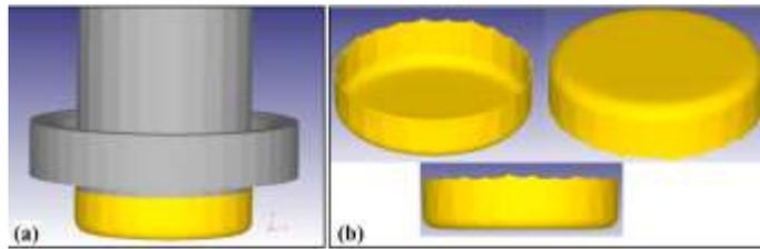
Fig -4: FE simulation of shallow-drawn cup (1st stage); (a) formed cup, (b) different views.
