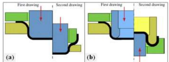
**Fig -1:** Two-stage deep drawing; (a) direct redrawing, (b) reverse redrawing [4].
