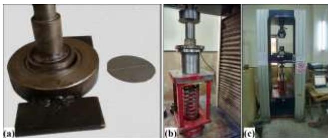
Fig -6: Drawing equipments; (a) cutting die for the blank, (b) tools with hydraulic press, (c) the entire setup.
