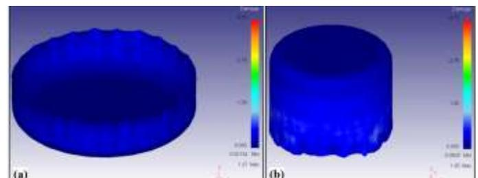
Fig -8: FE simulation of damage distribution for (a) shallow-drawn cup (1st stage), (b) reversely deep-drawn cup (2nd stage).
