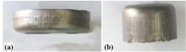
Fig -7: The produced cups; (a) Shallow-drawn cup (1st stage), (b) reversely deep-drawn cup (2nd stage).
