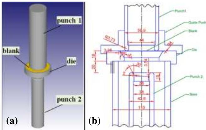
Fig -2: Parts assembly of deep drawing; (a) 3D view, (b) dimensional details.
