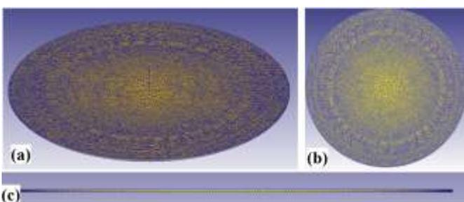
Fig -3: Meshing of the sheet metal; (a) 3D view, (b) Top view, and (c) side view.
