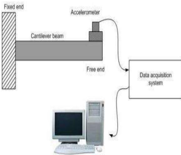
**Fig. 1:** An experimental setup for the free vibration of a cantilever beam
