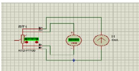
Figure -2: Implementation of RTD (4-wire Configuration)
