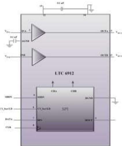
Figure -3: Block Diagram of PGA
