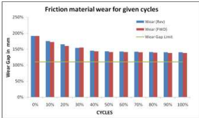
Fig.14 Synchronizer wear gap characteristics during durability test
