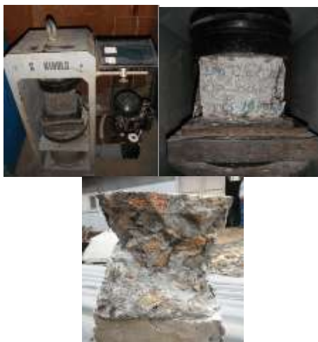
Fig 5.3 Compression Test Machine & Test Sample
