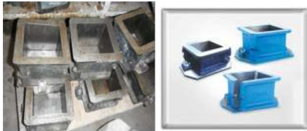
Fig 5.2 Typical 150 mm Cube Mould
