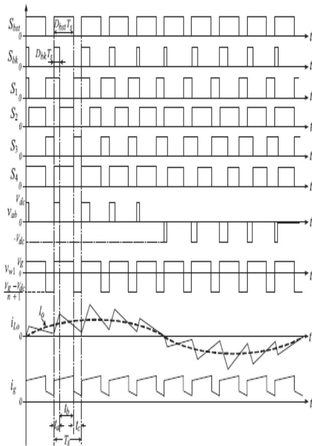
Fig-5: Key waveforms of the proposed SSBI topology [1]
