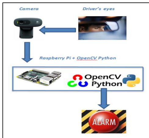
Fig -1: Proposed system architecture
