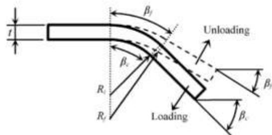
Fig 1:- Springback Effect in L Bending [12]
