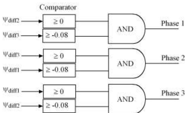
Fig-4: Commutation logic of the fixed turn-off angle method
