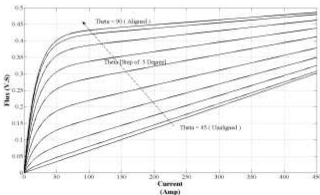
Fig-1: Magnetic Characteristics of 60KW 3-phase 6/4 pole SRM
