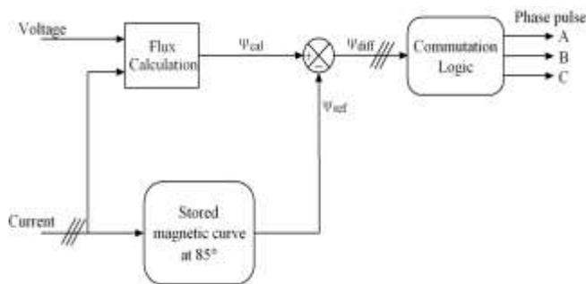
Fig-3: Block diagram of fixed turn-off angle method
