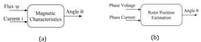
Fig-2: Basic block diagram of the flux-linkage based sensorless method
