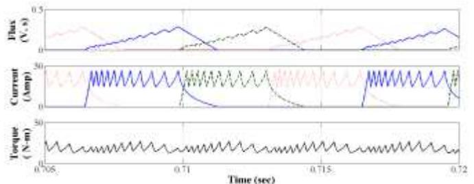
Fig-6: Waveform of the flux, phase current and torque at the speed of 1500 rpm
