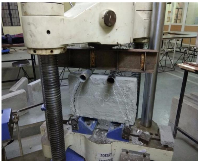
Fig 5.1 Flexural Test on UTM
