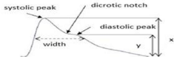
Fig 1: Typical PPG signal
