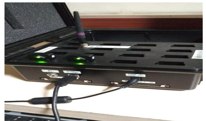
Fig -8: Trigno EMG wireless system with model SN: SP-W02A-1849
