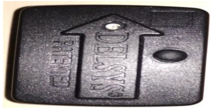
Fig -6: Wireless sensor used for the purpose of EMG measurement
