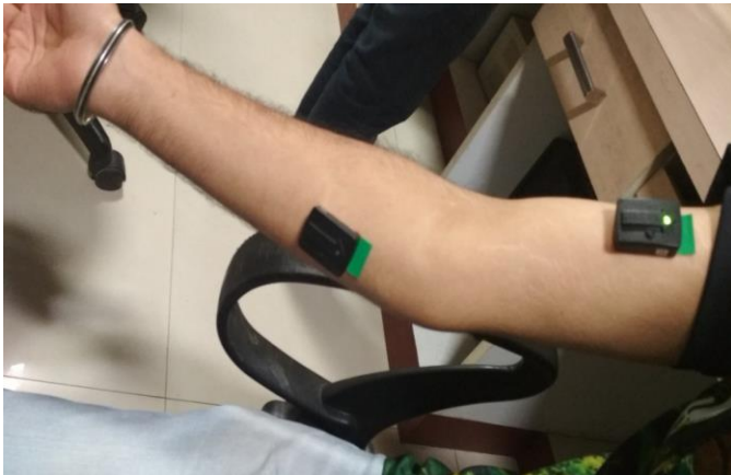
Fig -9: Sensors placed on both the concerned muscles using double-sided adhesive tapes.
