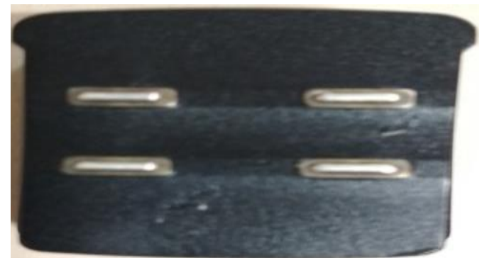
Fig -7: 4- channel Ag/AgCl electrodes used on the sensor
