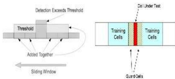
Figure 1.1: Cell - Averaging CFAR principle
