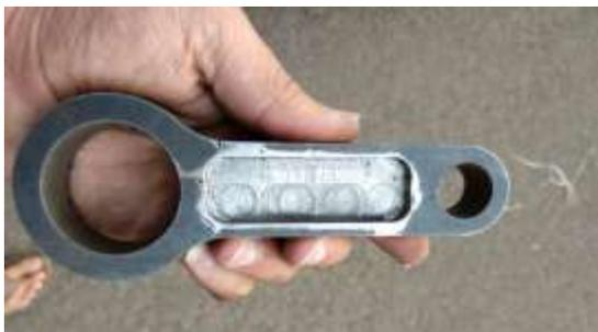
**Fig11:** Fabricated connecting rod according to optimized dimensions
