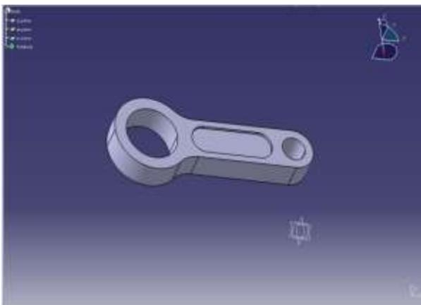
Fig 3: Reversed cad developed design of connecting rod
