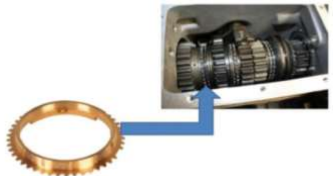
Fig -3: Synchronizer ring GBS 40
