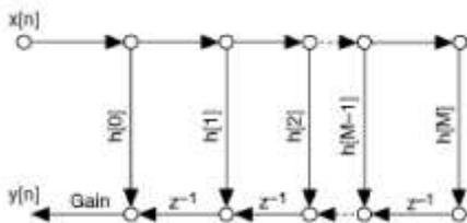
Figure 3: Transposed Form Realization of FIR Filter
