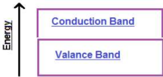
Fig-3:- Energy band diagram of Conductor
