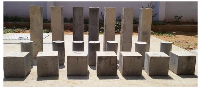
Fig -5: Demoulded and cured specimens at 28 days
