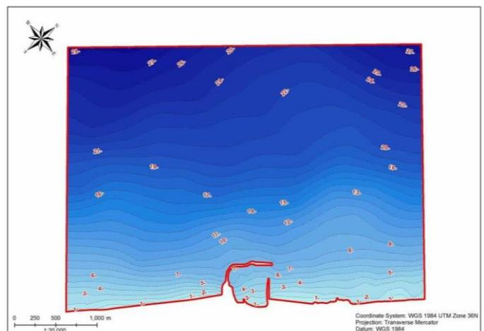
Fig -1: The bathymetric features of the Gaza fishing port
