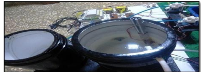
Fig .2.2.1 Water level sensor/detectors
