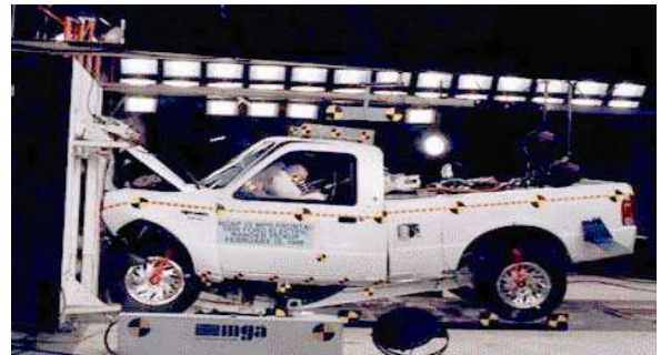
Figure 11: Frontal Impact Crash Test.
