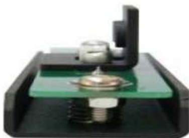
Fig.2: Sensor assembly of the car bumper
