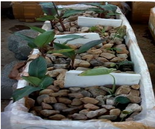
Fig -1: Constructed Phytotechnology reactor.
