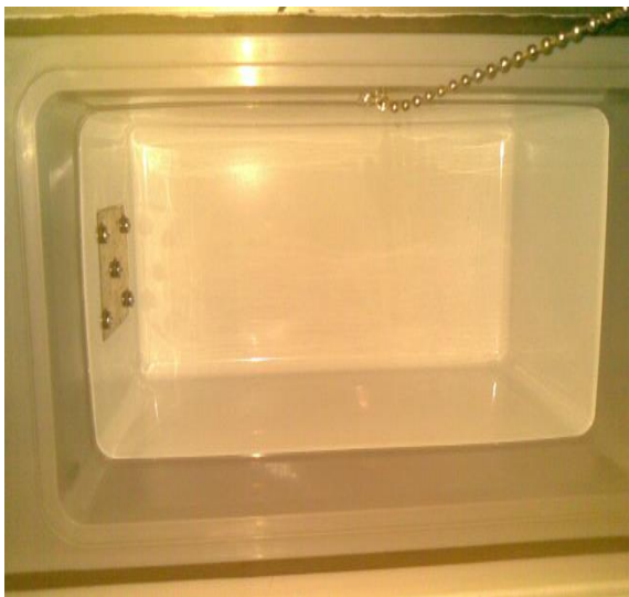
Fig-8: Insulated Chamber of Peltier Cooler
