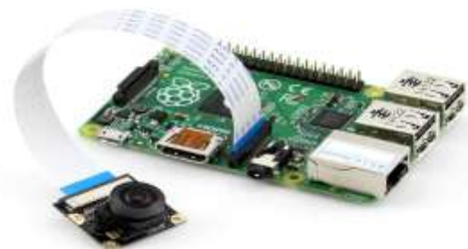
Fig 1: Raspberry Pi with Pi Camera Attached
