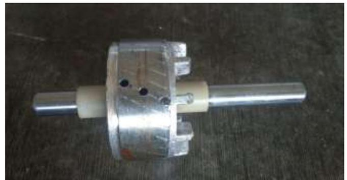
Fig.-2 Broken Rotor Bar
