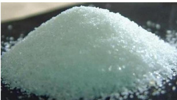
**Fig 1** - Powdered form of Super Absorbent Polymer – SAP
