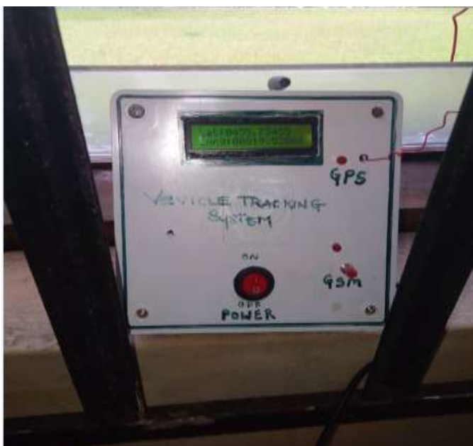
Fig - 4: Image of the complete system assembly with LCD showing the location of the vehicle
