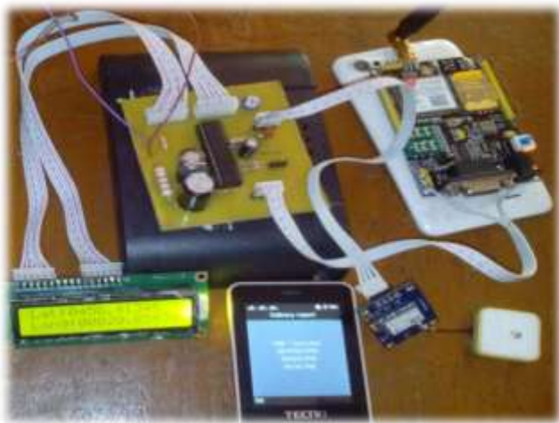
Fig-3: Image of the complete system assembly with LCD showing the position of the vehicle
