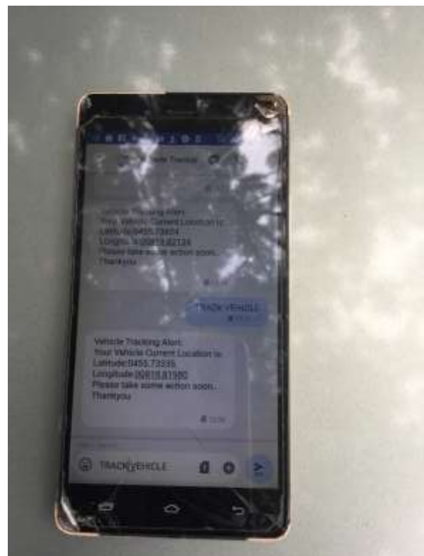
Fig-5: Owner's mobile phone Screenshot of returned SMS to a TRACK VEHICLE request
