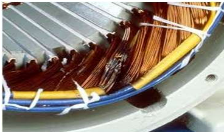
Fig:1 A faulty electric motor winding
