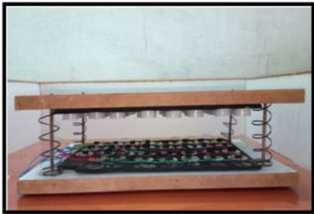
Fig -10: Final piezo material arrangement
