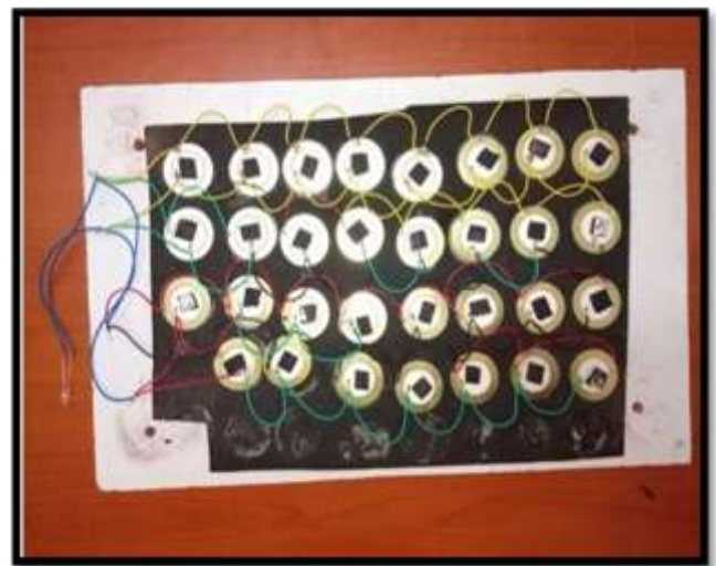
Fig -8: Series and Parallel Connection Arrangement
