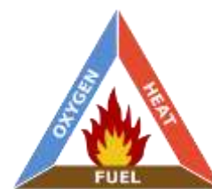
Fig -2: The Fire/Combustion Triangle
