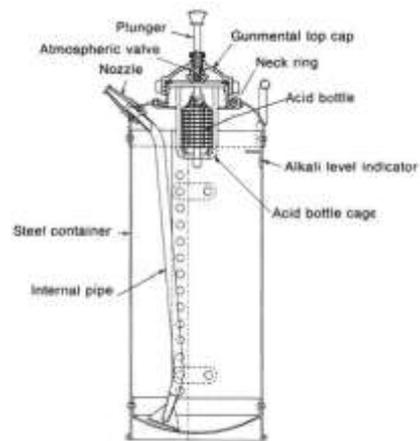
Fig -10: Wet Chemical Fire Extinguisher [10]
