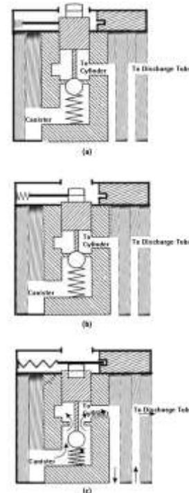
**Fig -14:** Proposed Two-Stage Push Button Discharge Mechanism
