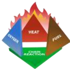
Fig -3: The Fire/Combustion Tetrahedron
