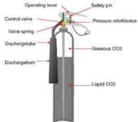
Fig -9: Carbon-dioxide Fire Extinguisher [10]
