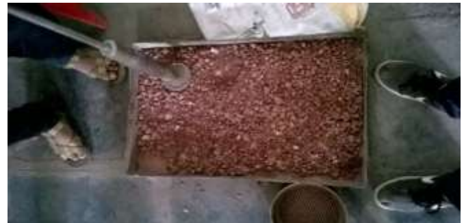
Figure -1: Crushed laterite stone
