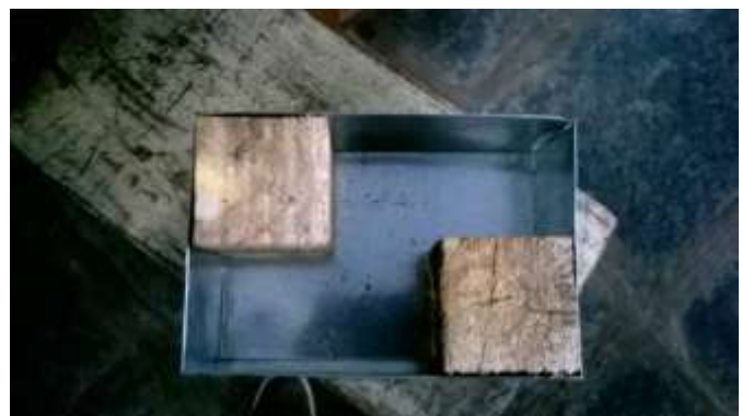
Figure -2: Fabricated Z-shape mold
