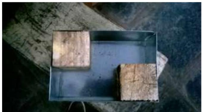
**Figure -2:** Fabricated Z-shape mold
