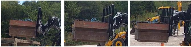
Fig. 15 Strain gauge testing of inner boom [Source: Testing report]
