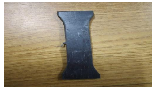
Figure 4.18: Compression specimen after testing
