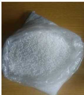
Figure 3.3: High Density Polyethylene
