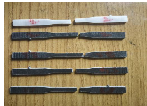
Figure 4.15: Tensile specimen after testing in UTM
