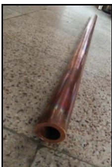
Fig 1 It is smooth (plane) tube. Tube has dimension I.D. 25mm, O.D. 38mm and 1m in length.
