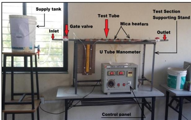
Figure 2.1.1: Experimental Setup
