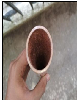
Fig 1 It is smooth (plane) tube. Tube has dimension I.D. 25mm, O.D. 38mm and 1m in length.
