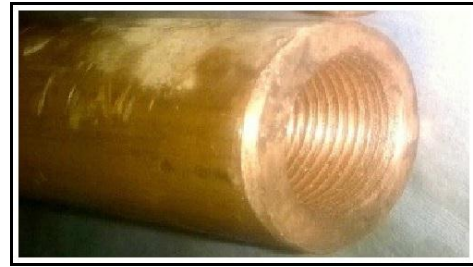
Fig 3 It is threaded tube have pitch 4mm.
