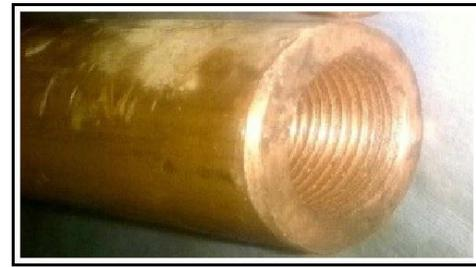
Fig 3 It is threaded tube have pitch 4mm.
