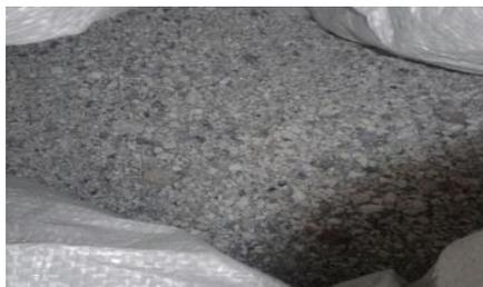
Fig-2: Steel Slag
