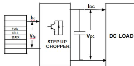
Fig.1. Block diagram of fuel cell power system
