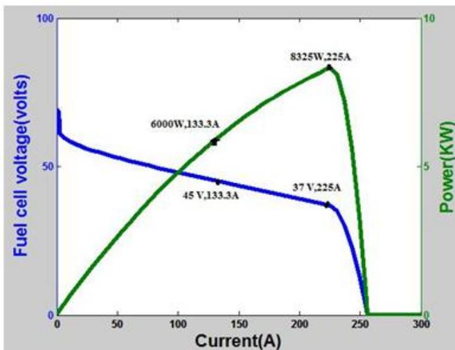
Fig.3. V-I and P-I characteristics of fuel cell
