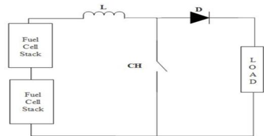
Fig.6: Fuel Cell Power System
