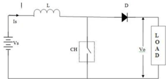
Fig.4. Circuit diagram of step-up chopper
